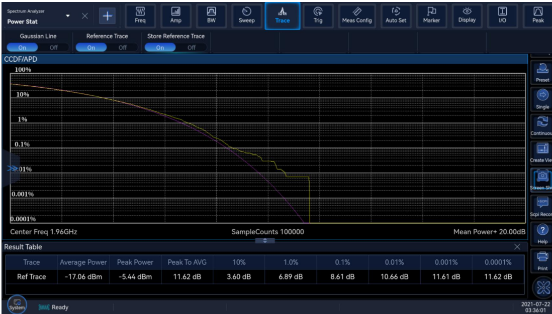
Figure 4.18 Storing and displaying CCDF measurements
