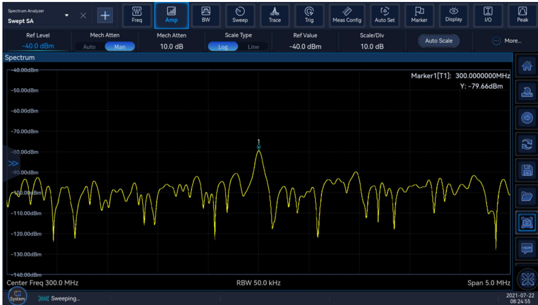
Figure 4.4 Small signal at 10dB of the attenuator by default
