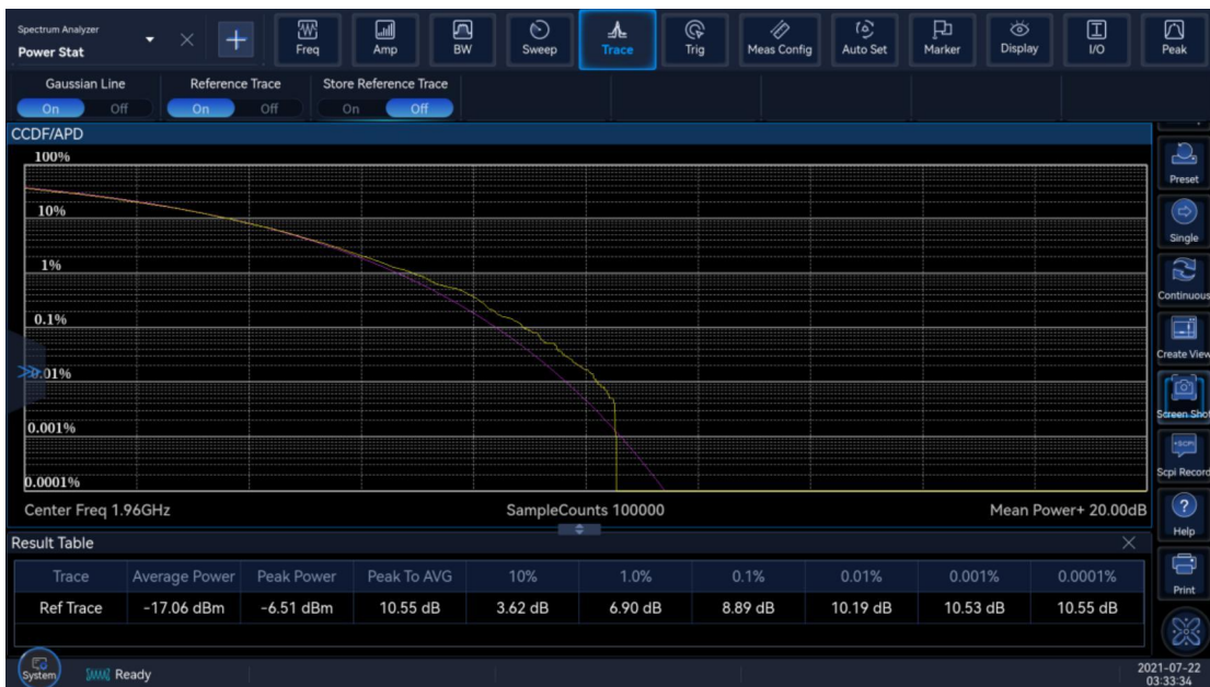
Figure 4.17 Power statistics measurement result
