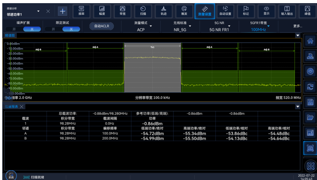
2GHz carrier 5G NR ACPR measured value
