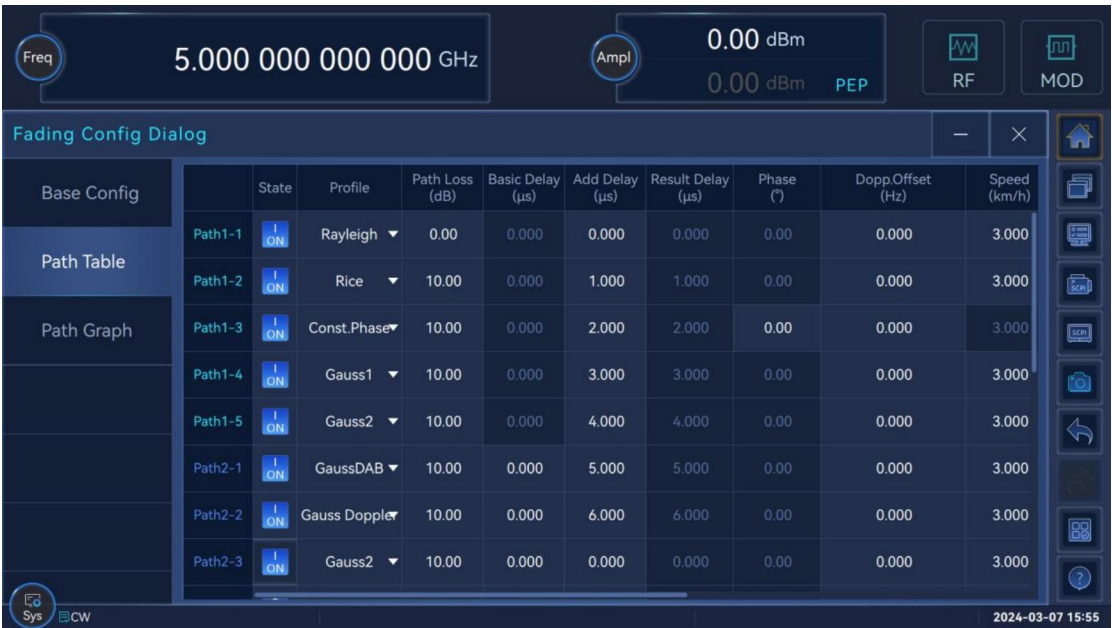
Real-time fading simulation configuration interface
