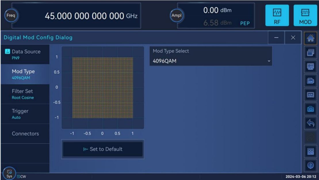
4096QAM modulation configuration interface
