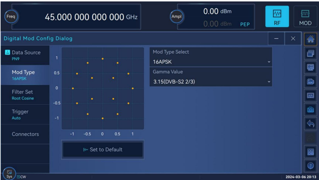
16APSK modulation configuration interface
