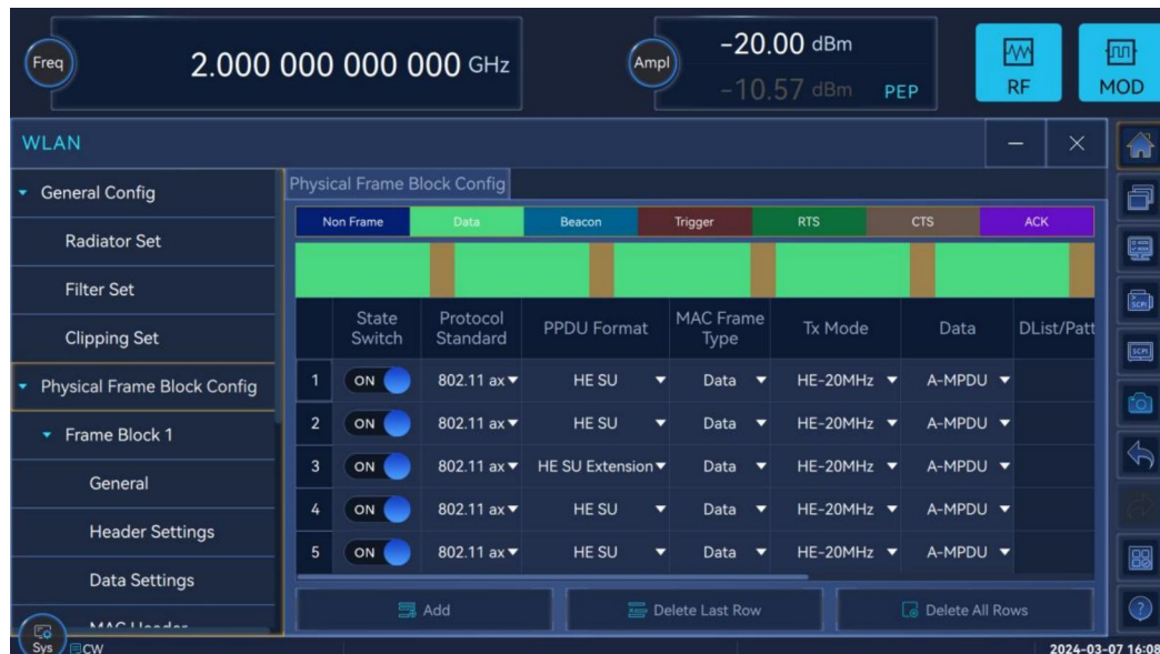
WLAN physical frame block configuration interface
