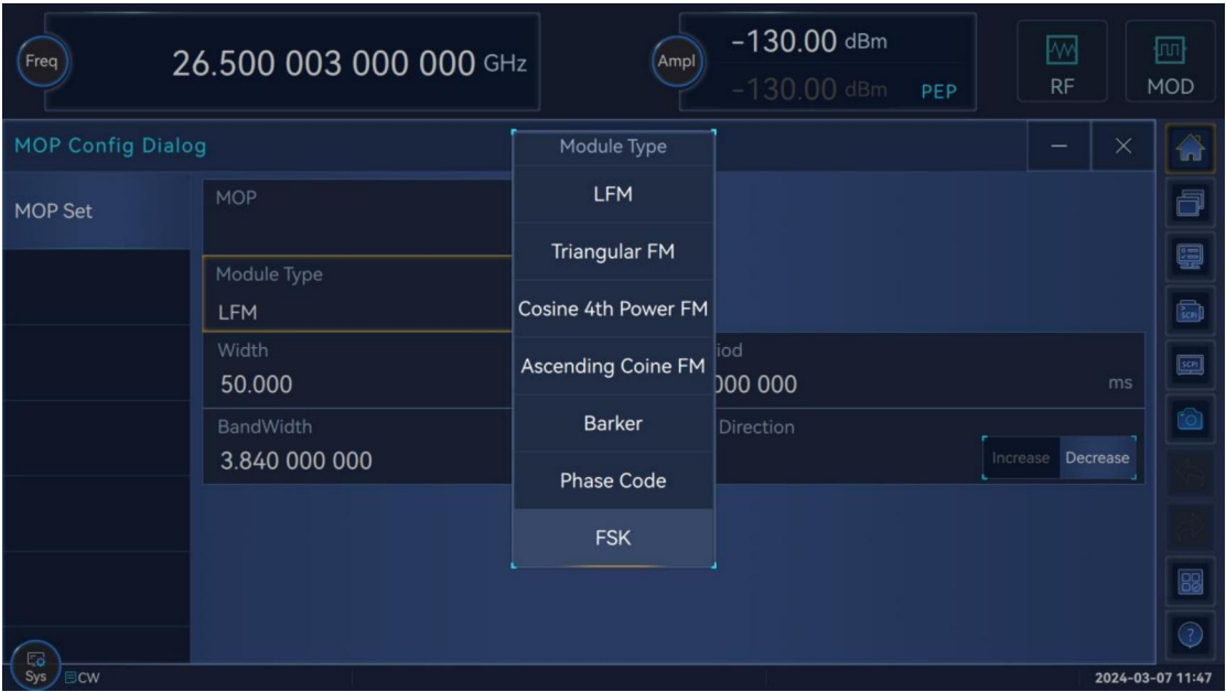
Intrapulse modulation configuration interface
