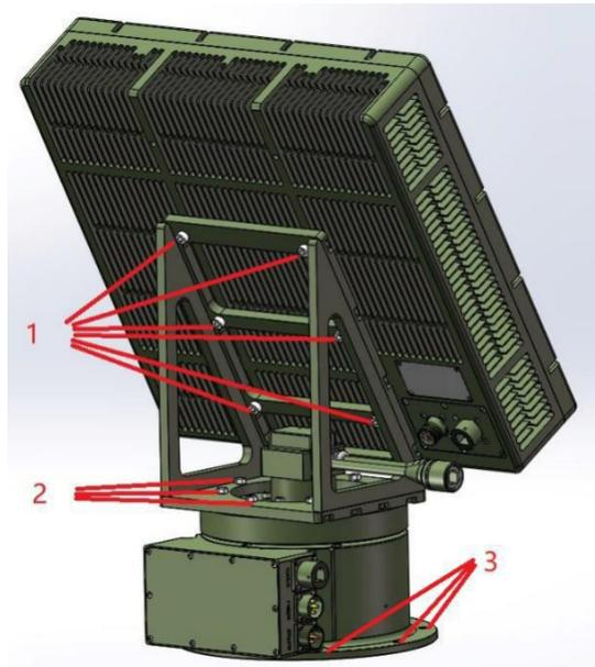
Figure 2.4 Screw mounting position diagram
