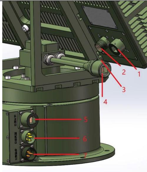
Figure 2.3 Radar interface diagram
