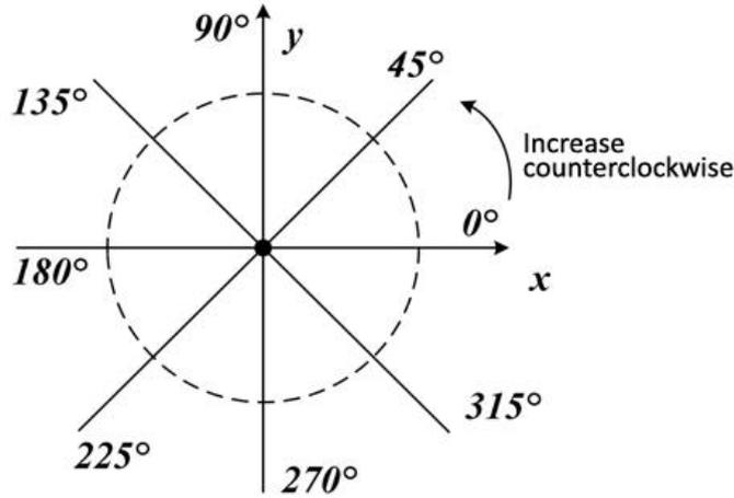
Figure 3.7 Radar coordinate system
