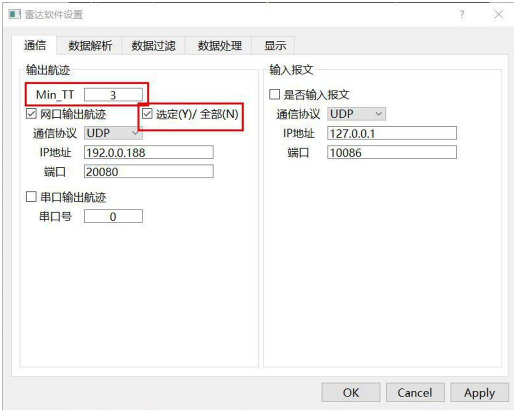
Figure 3.10 Select track or all output diagram
