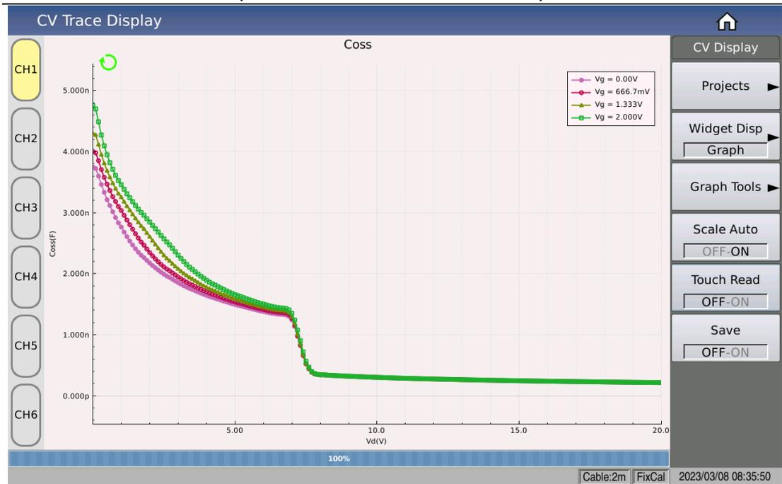
(Figure 3-5-5 Trace Coss Model Scan Graphic Display)
