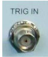
Fig. 3-21 External Trigger Input Connector
