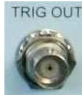
Fig. 3-22 External Trigger Output Connector
