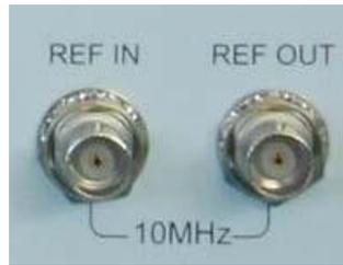
Fig. 3-15 10MHz Reference Connector
