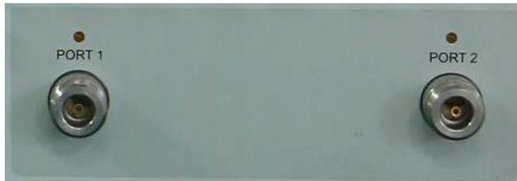
Fig. 3-13 Measure Ports of the Analyzer
