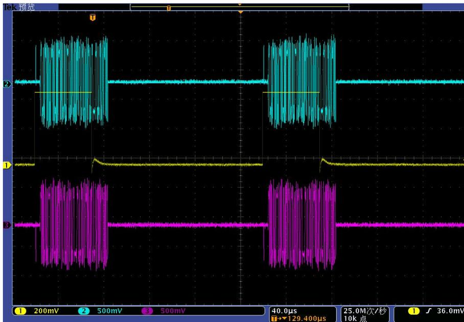
Figure 3.23 Baseband triggering (Continuous/Single)
