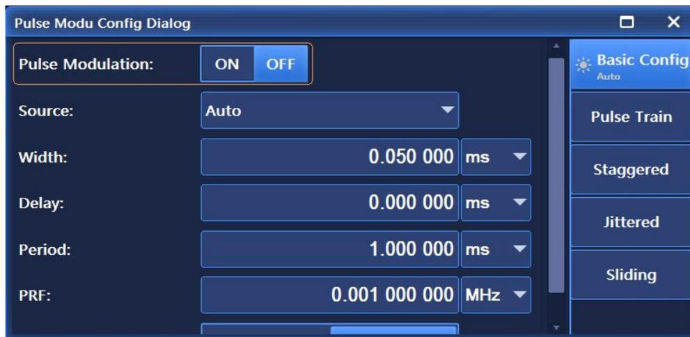
Figure 4.19 Pulse Modu Config interface
