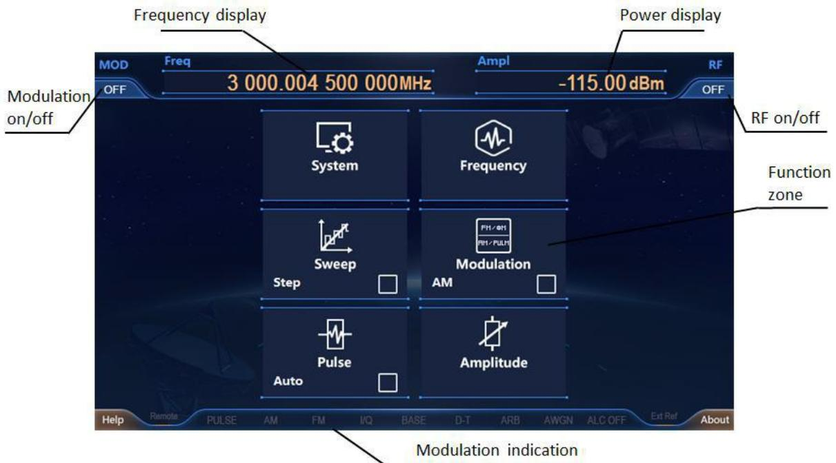
Figure 2.13 Operator interface of S1435
