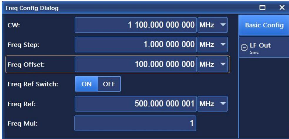
Figure 2.18 Setting frequency offset to 100MHz
