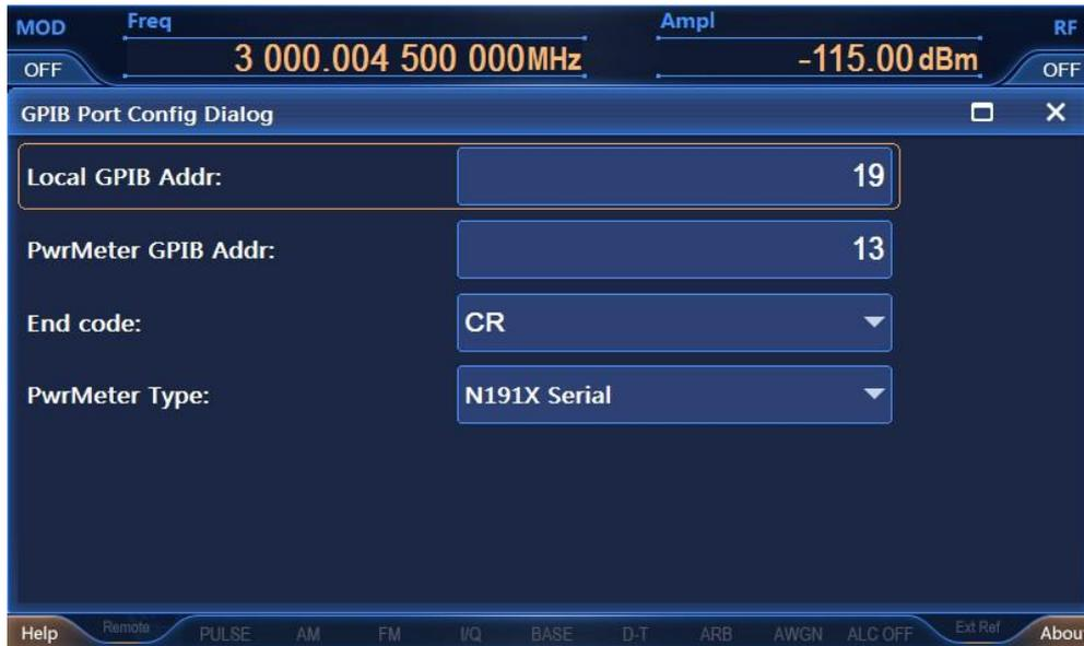
Figure 2.9 GPIB port setting
