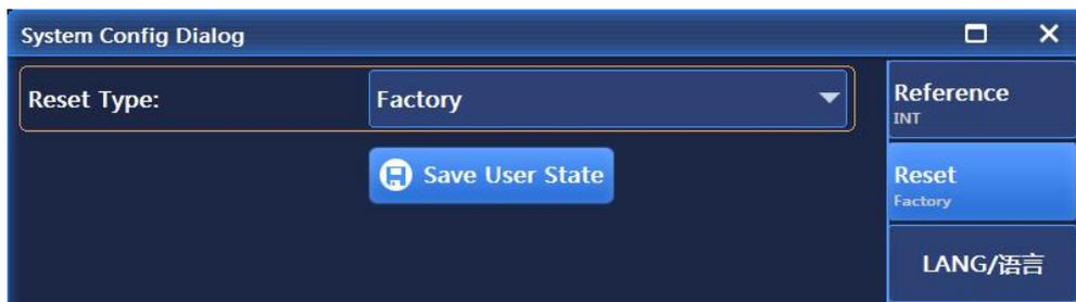
Figure 2.47 Setting reset state
