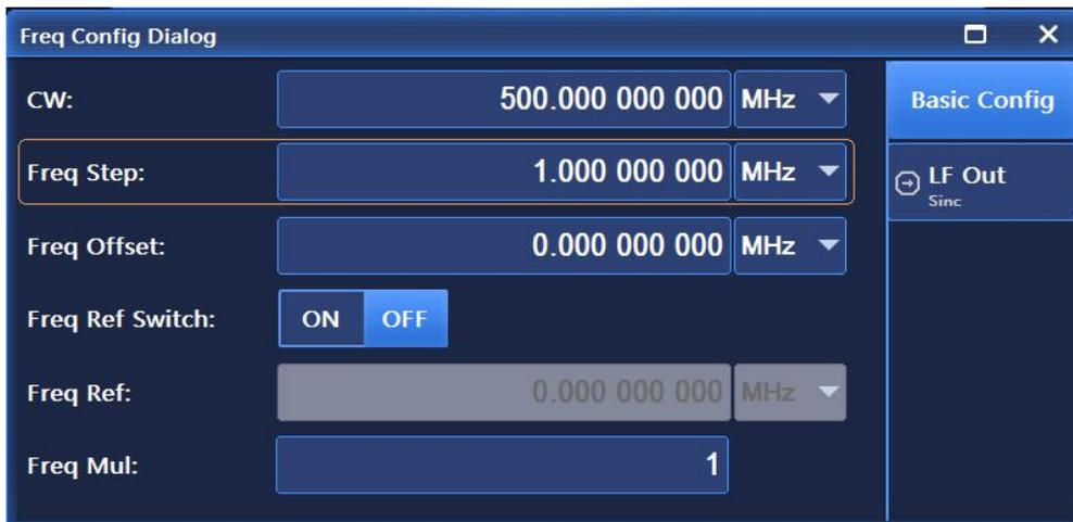
Figure 2.16 Setting the continuous wave to 500MHz, frequency step to 1MHz and a step frequency
