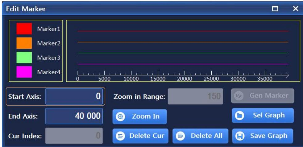
Figure 3.11 Setting waveform segment marker
