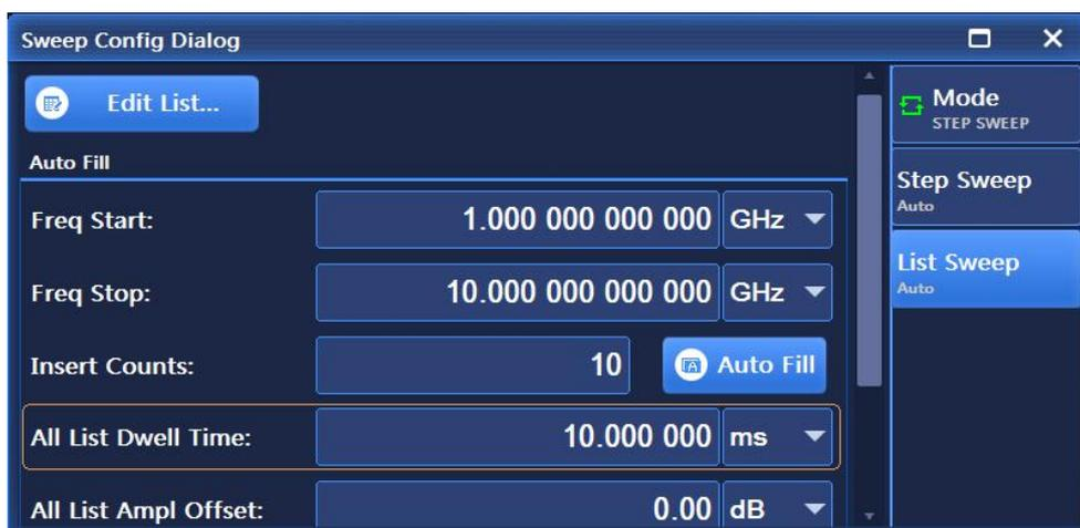
Figure 3.6 List sweep configuration window
