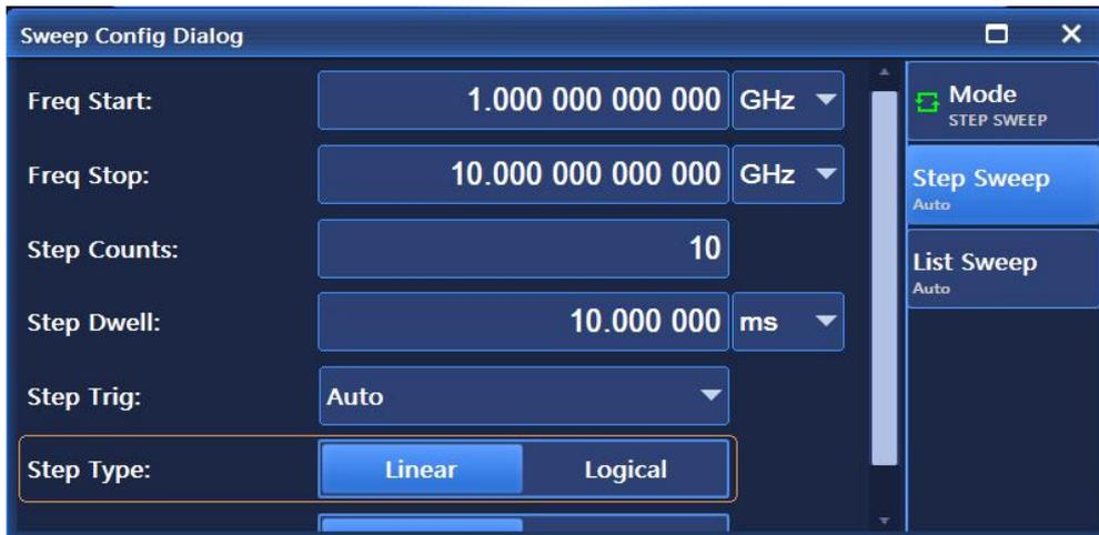
Figure 3.5 Step sweep configuration window
