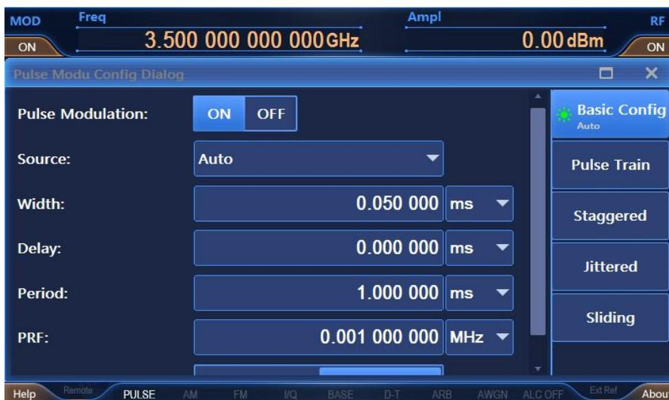
Figure 2.23 Setting pulse modulation signals
