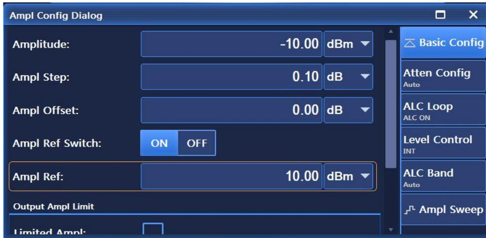
Figure 2.20 Power 0dBm, power reference 10dBm
