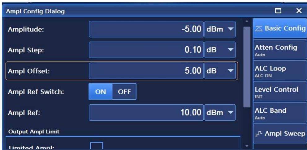
Figure 2.21 Power offset set to 5dB
