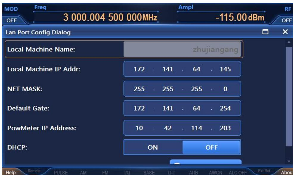
Figure 2.10 LAN port configuration
