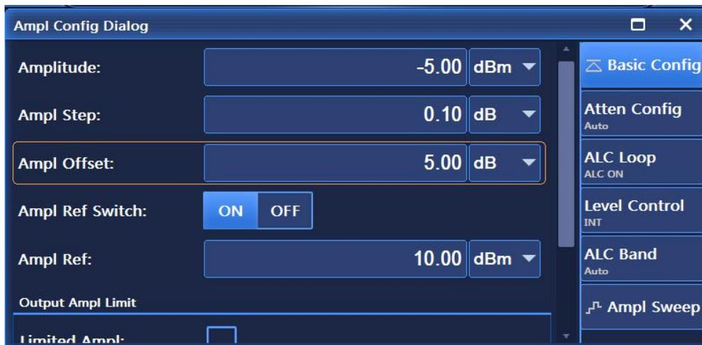
Figure 2.21 Power offset set to 5dB
