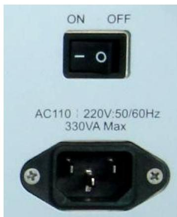
Fig. 4-25 Power Socket and Power Switch
