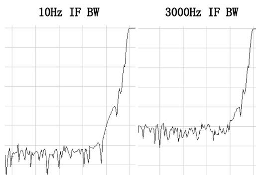
Fig. 6-12 Influence on Measure Result from Intermediate-frequency Bandwidth
