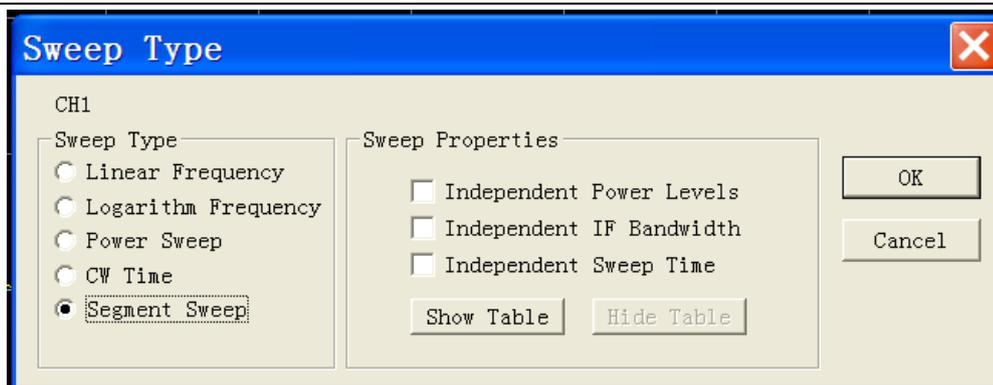
Fig.5-16 Setup of Segment Sweep Type
