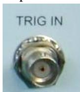
Fig. 4-23 External Trigger Input Connector
