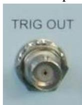
Fig. 4-24 External Trigger Output Connector
