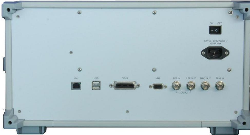
Fig. 4-16 Analyzer Rear Panel
