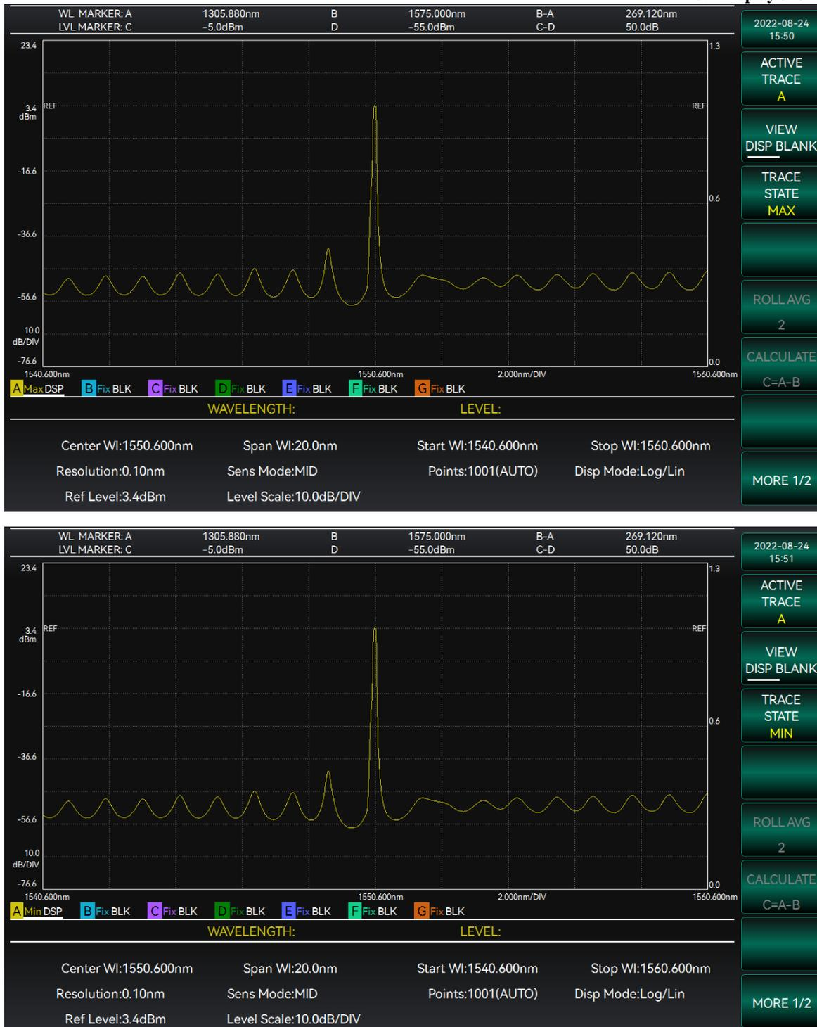
Figure 3-32 Curve hold condition diagram
