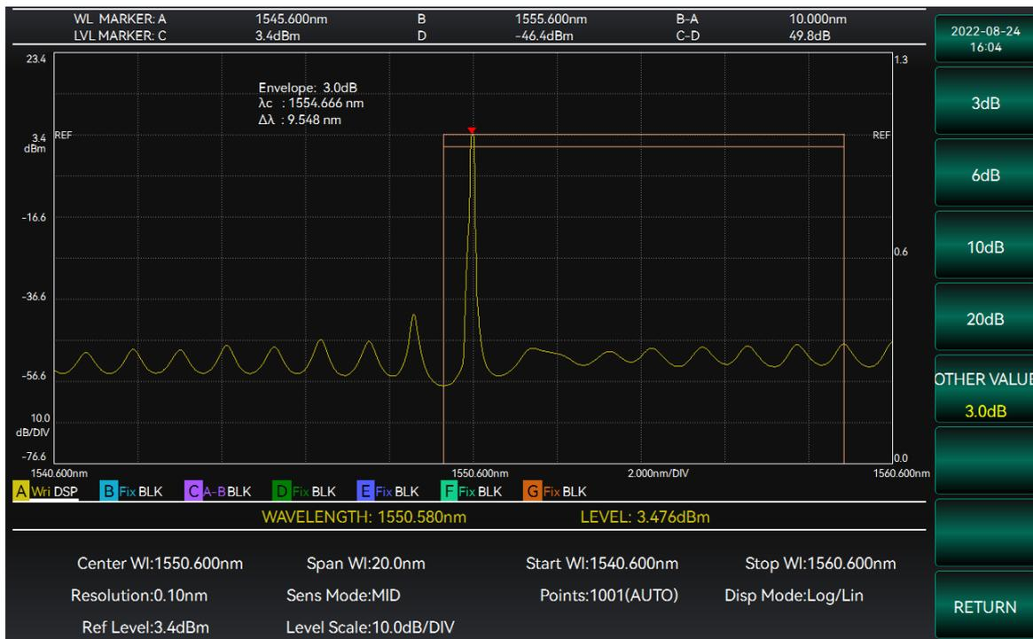
Figure 3-48 Envelope analysis interface diagram
