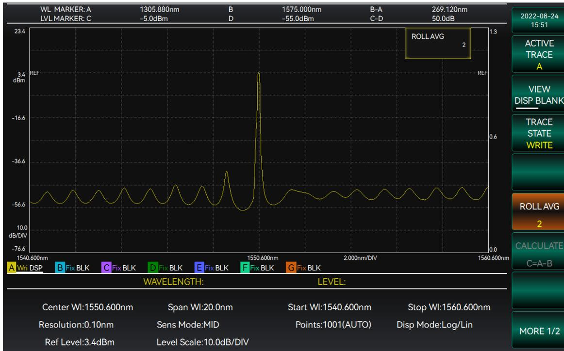
Figure 3-33 Setting curve weighted average diagram
