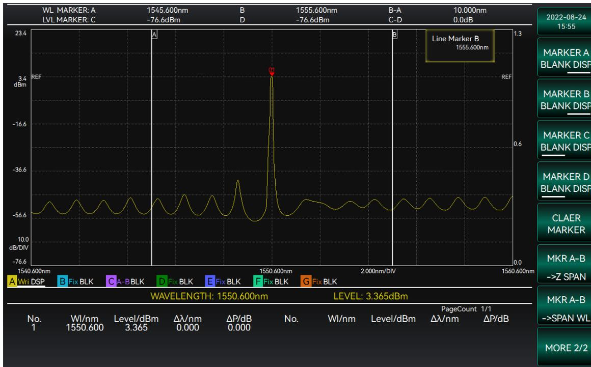
Figure 3-38 Setting markers A and B diagram
