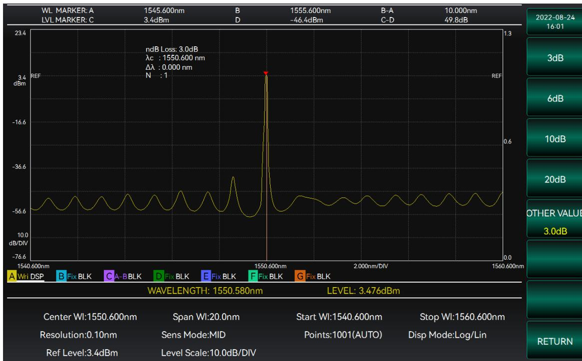
Figure 3-46 ndB loss analysis interface diagram
