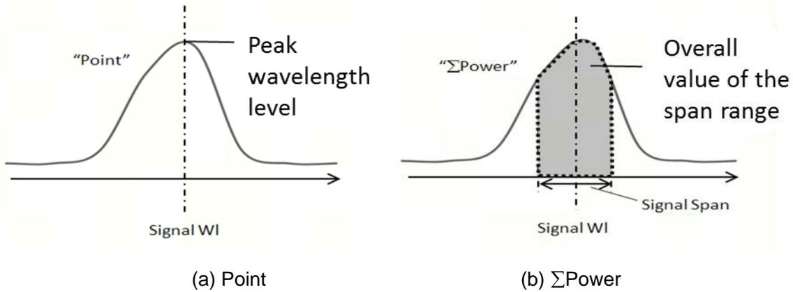
Figure 3-65 Schematic diagram of signal power measurement method
