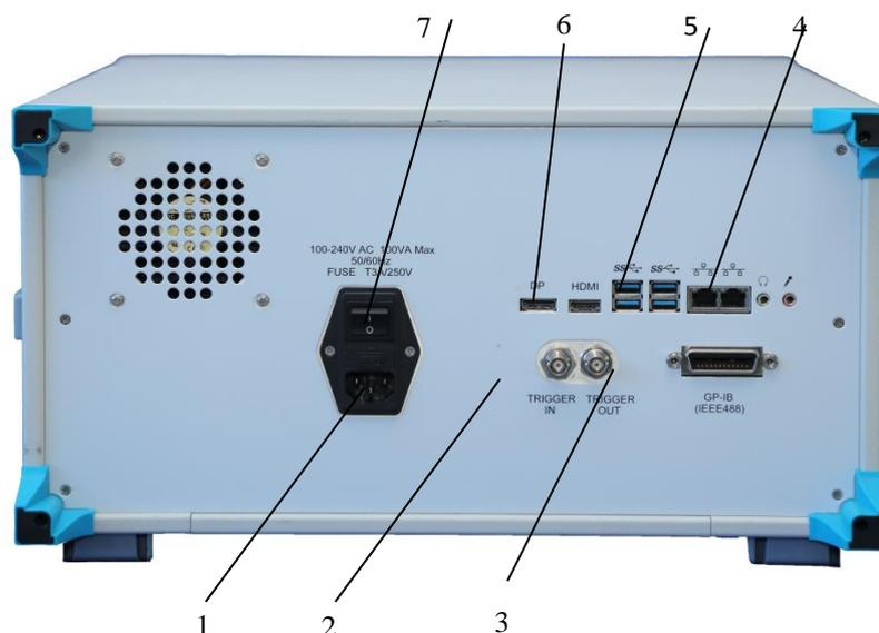
Figure 3-7 Rear panel of S6362D optical spectrum analyzer
