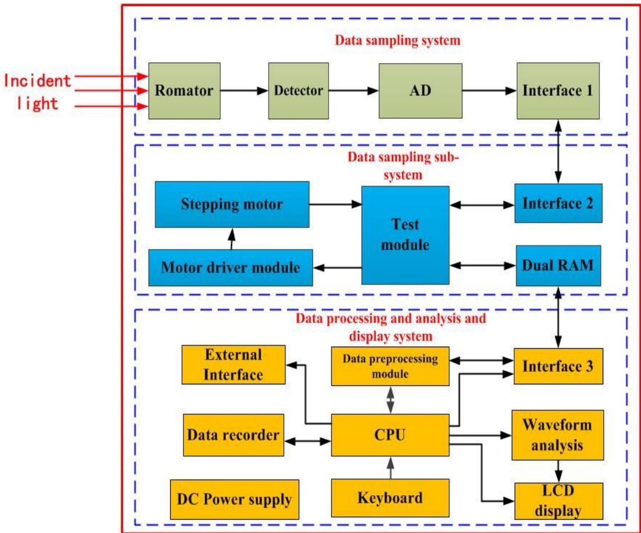
Figure 4-1 Block diagram of overall analyzer scheme
