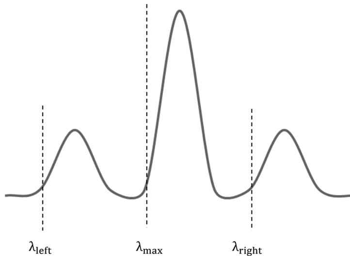
Figure 3-59 Schematic diagram of side mode wavelength symbols
