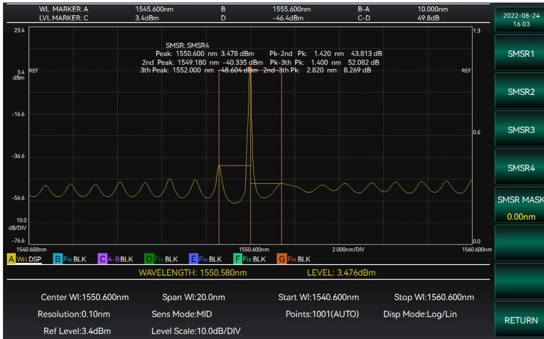
Figure 3-47 SMSR analysis interface diagram
