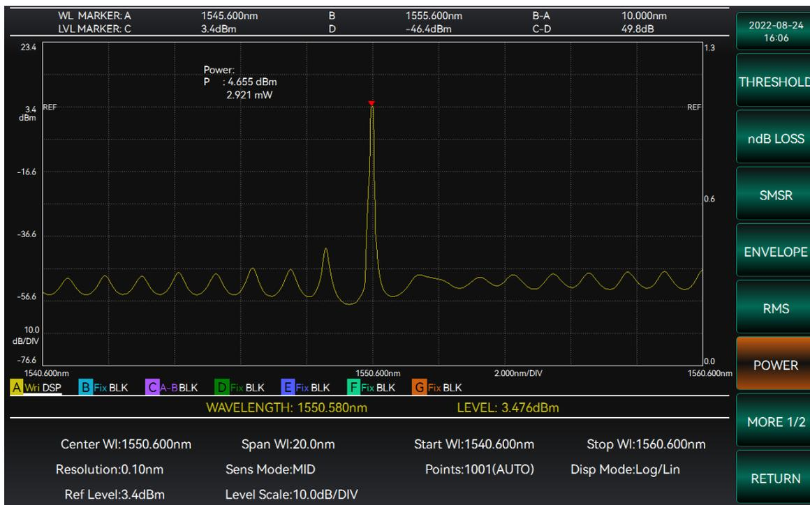
Figure 3-50 Spectral power analysis interface diagram
