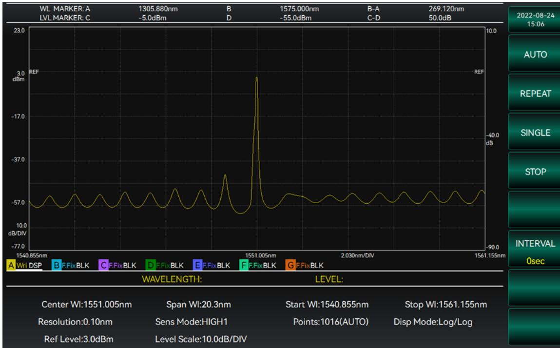
Figure 3-8 Operation interface of S6362D optical spectrum analyzer
