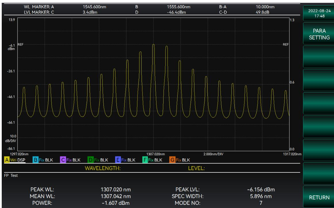
Figure 3-55 FP-LD test interface diagram
