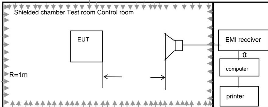
Figure 3.15 Schematic diagram of RE102 measurement
