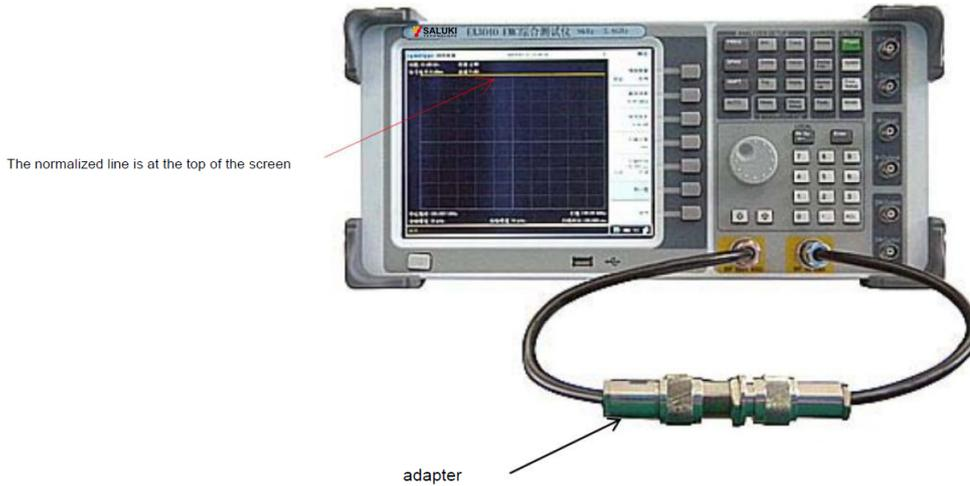
Figure 3.29 Normalized measurement
