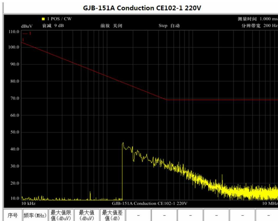
Figure 2.3 EMI receiver CE102 operation interface
