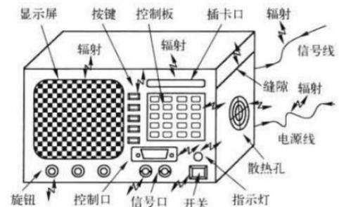
Figure 4.1 Measuring Electromagnetic Emissions from Equipment with Near Field Probes
