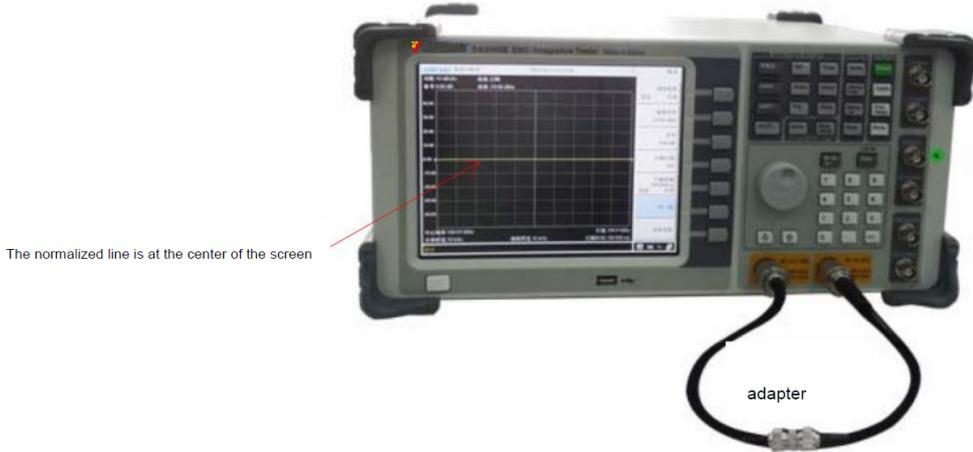
Figure 3.28 Normalized measurement
