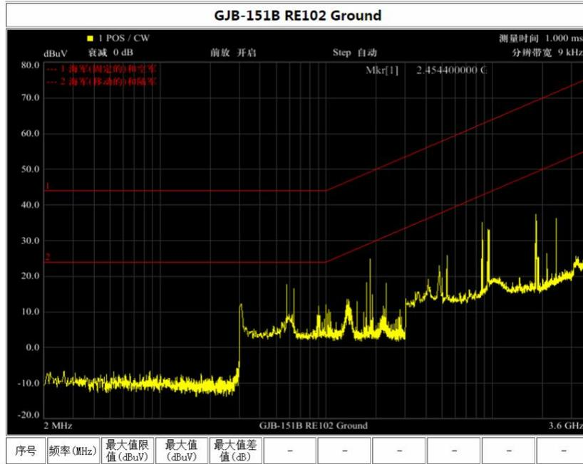
Figure 3.16 GJB151B RE102 test interface
