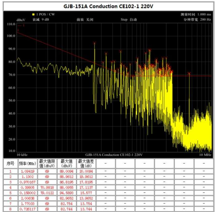
Figure 3.14 Test report and list of out-of-standard points
