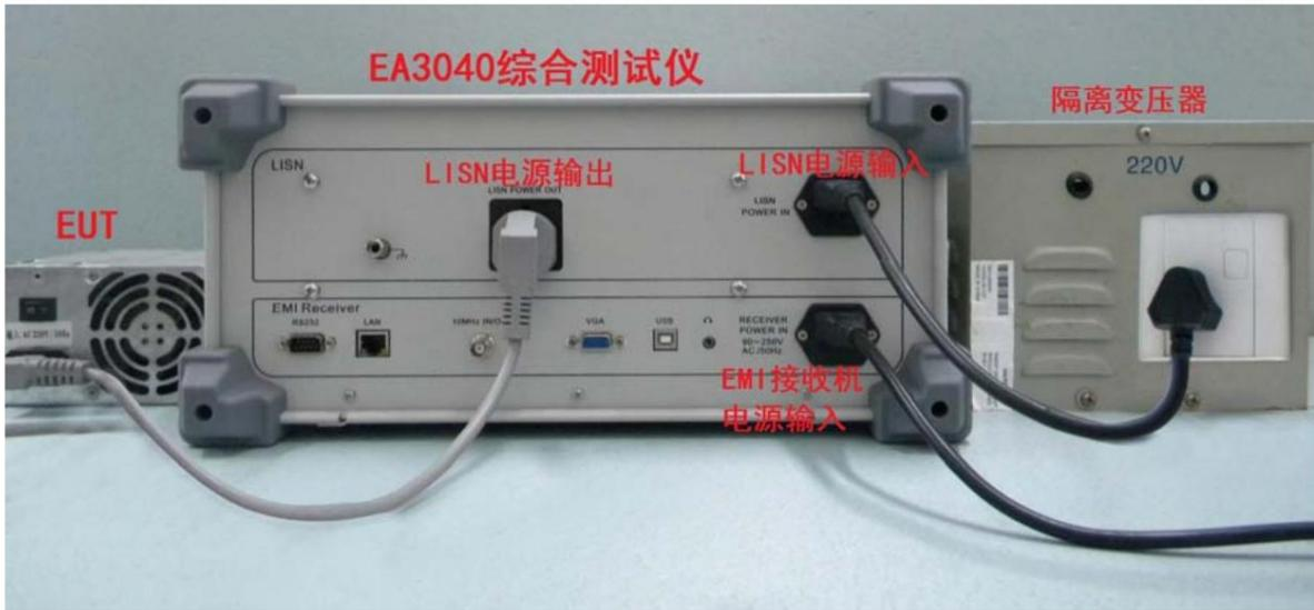
Figure 4.7 Connection Diagram of CE102 Conduction Test Example
