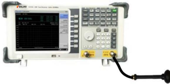
**Figure 4.2** Measuring electromagnetic radiation of PCB board with near-field probe
