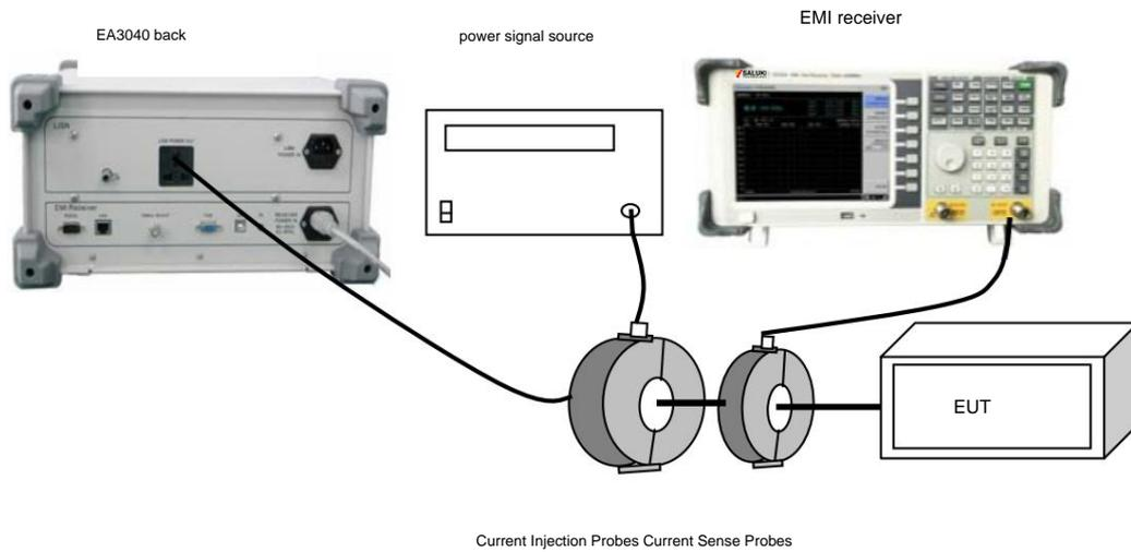
Figure 4.6 Sensitivity measurement by current injection method
