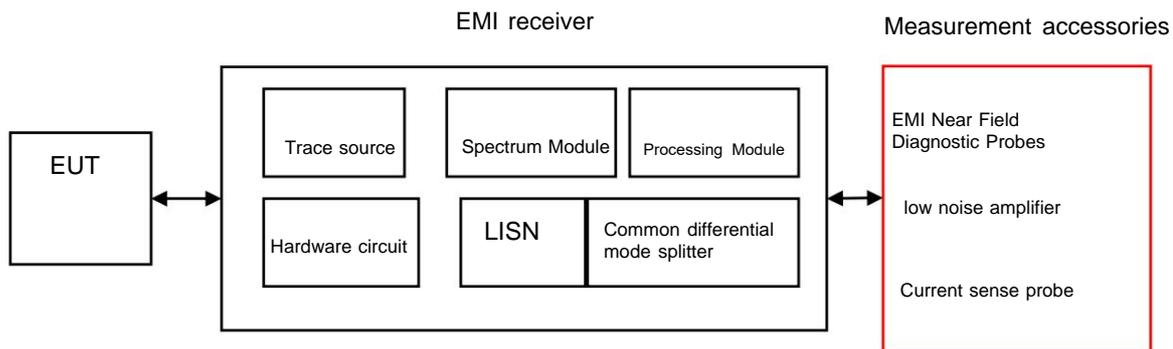
Figure 1.2 EMI receiver measurement block diagram
