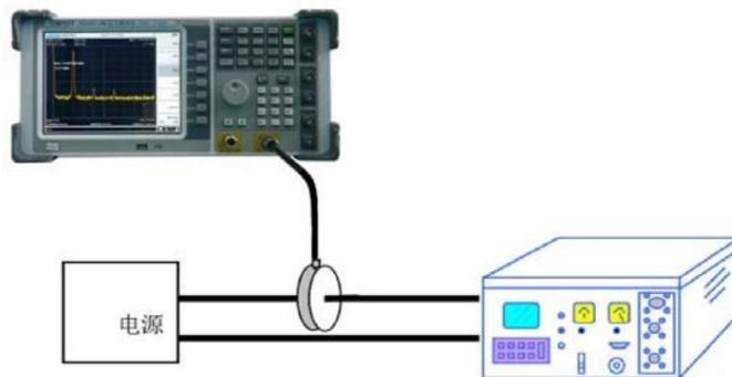
Figure 4.4 Current detection probe measures interference on power and signal lines
