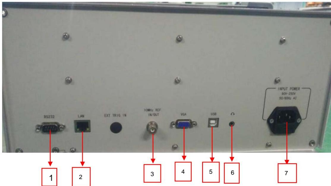
**Figure 1.4** ER series EMI receiver rear panel
