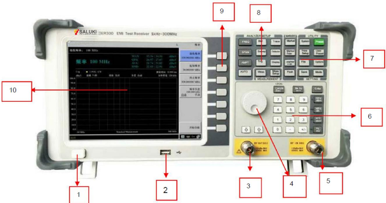
Figure 1.3 Front panel of ER series EMI receiver
