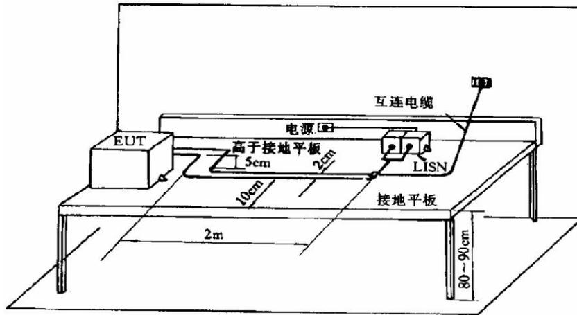
Figure 3.20 CE102 test block diagram and specifications
