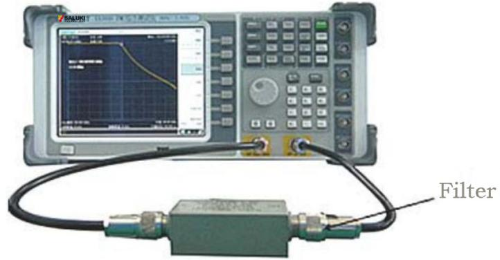
Figure 3.30 Filter measurement
