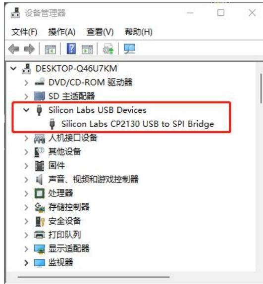
Fig. 6 Check whether the LSG022 is correctly identified in “Device Manager”
