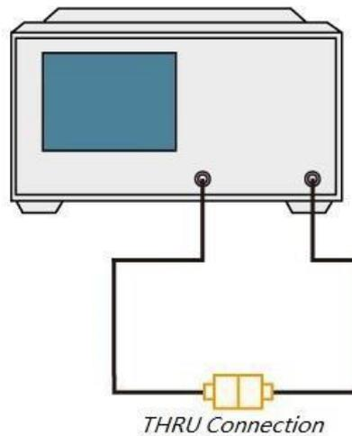
Figure 3-9 Transmission Response Calibration - DUT Connection Diagram
