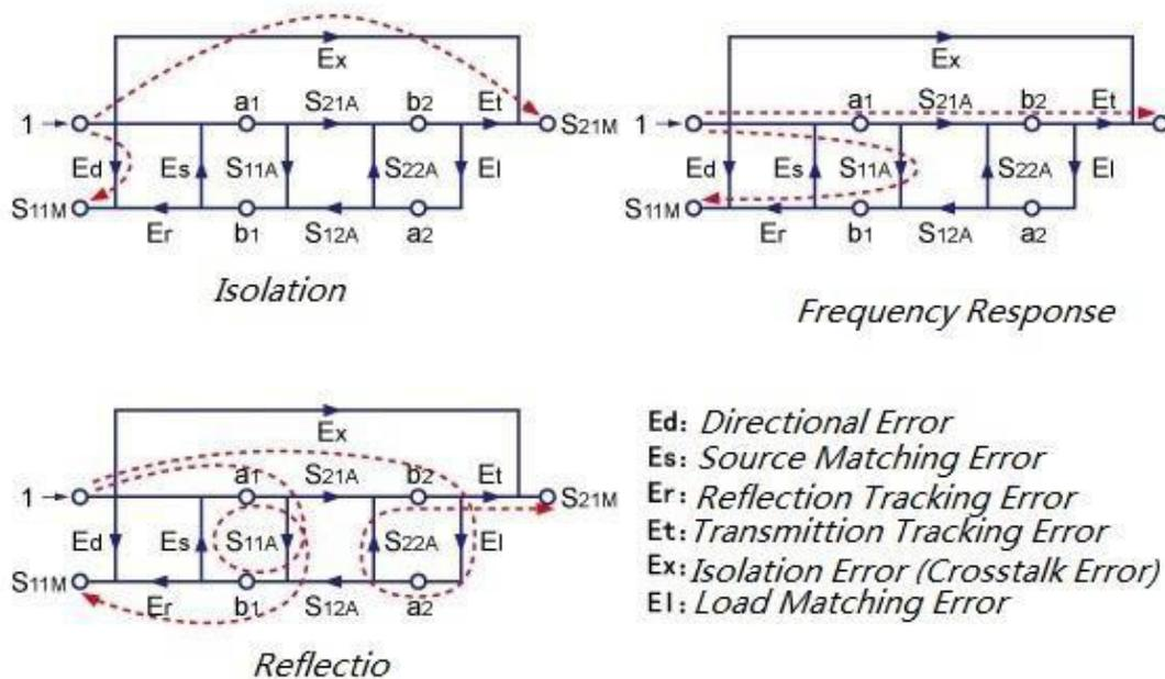
Figure 3-14 All 2 port calibration - 12 error
