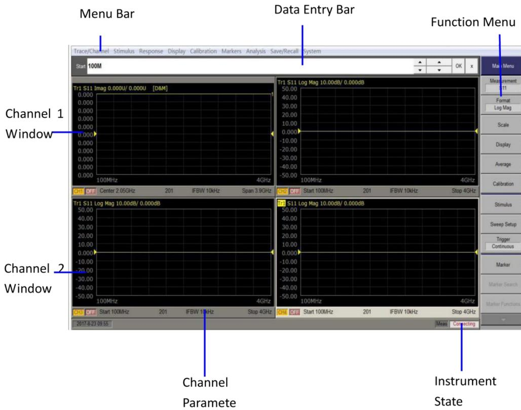
Figure 1-3 Instrument Display Interface
