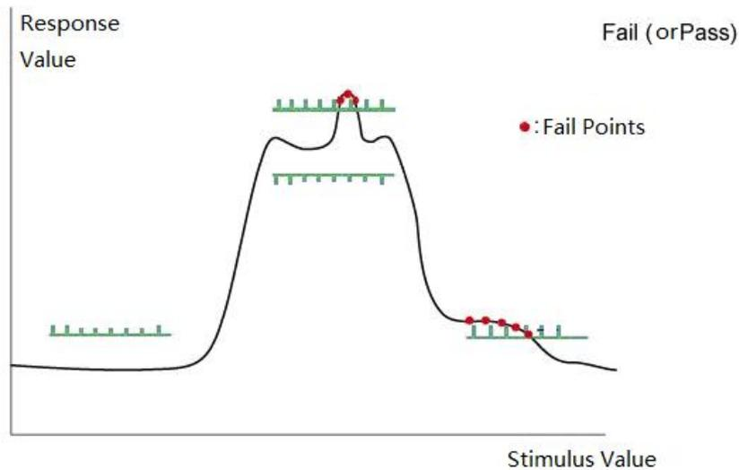
Figure 5-22 Limit test schematic
