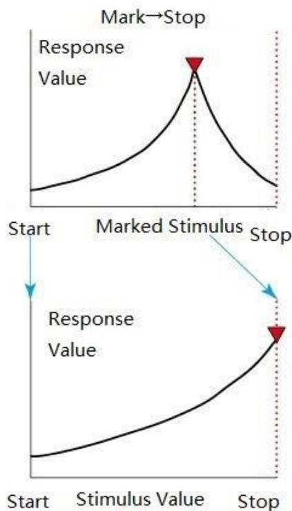
Figure 5-17 Marker Transfer --- Marker -> Stop Function
