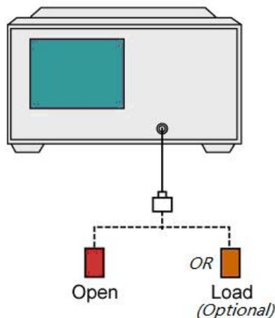
Figure 3-5 Open Response Calibration - DUT Connection Diagram
