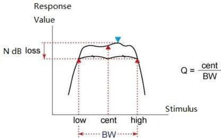
Figure 5-12 Bandwidth Search Parameter Definition--- Bandpass Filter
