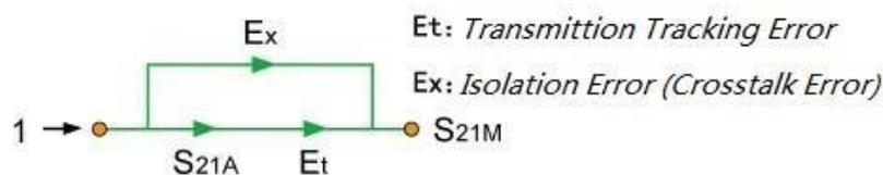
Figure 3-8 Transmission Response Calibration (Direct Response + Isolation)
