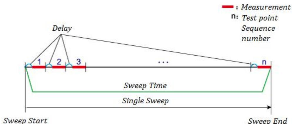
Figure 2-3 Measurement delay diagram
