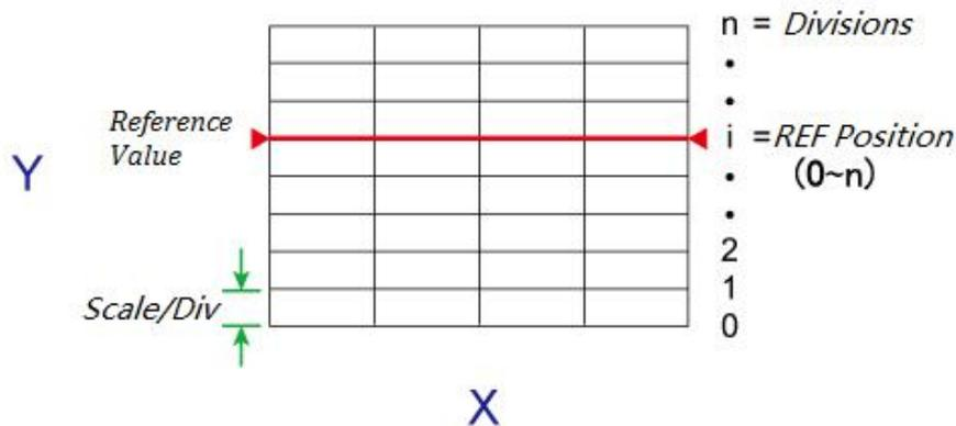
Figure 2-7 Manual adjustment Cartesian scale
