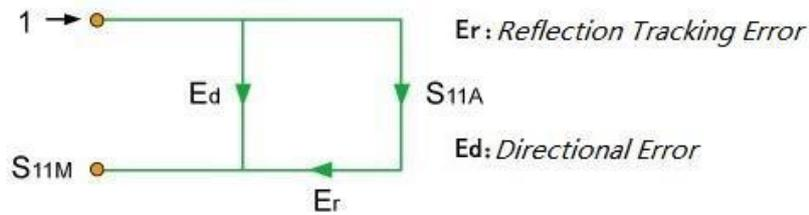
Figure 3-4 Open-circuit response calibration (open-circuit response + isolation)
