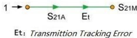
Figure 3-7 Transmission Response Calibration (Direct Response)
