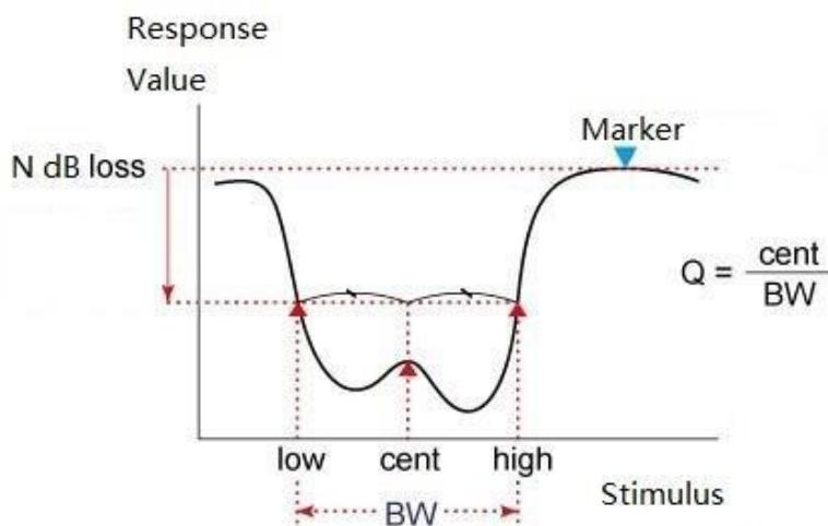
Figure 5-12 Bandwidth Search Parameter Definition---Bander Filter
