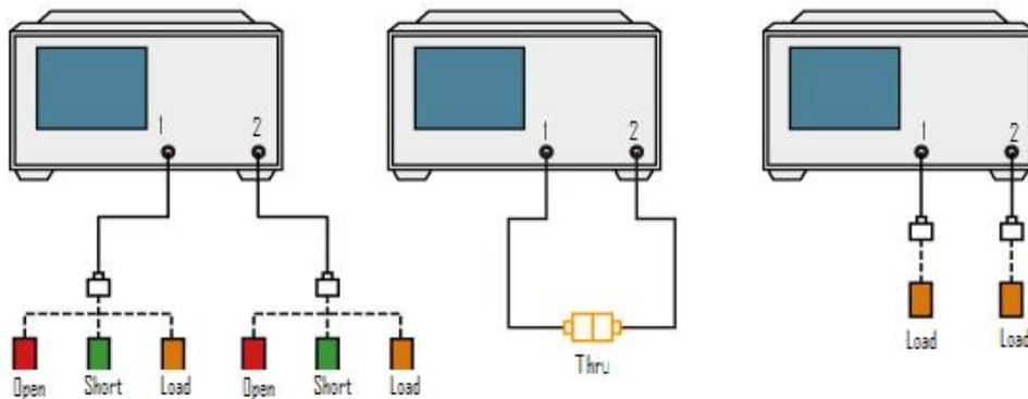
Figure 3-15 Full 2-port calibration - Calibration section connection diagram
