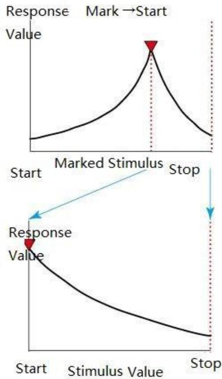
Figure 5-16 Marker Transfer --- Marker -> Start Function
