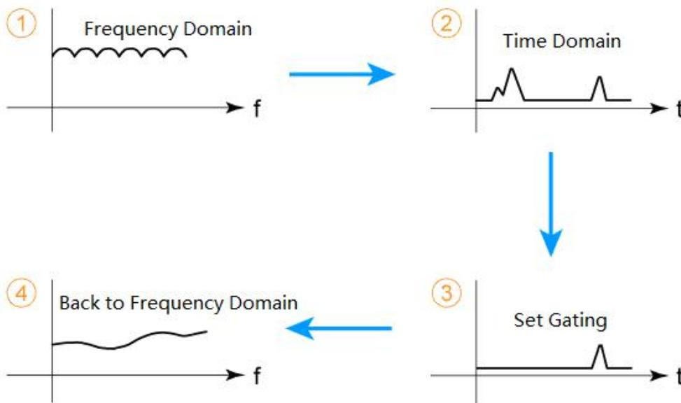
Figure 5-30 Time domain gating measurement flow diagram
