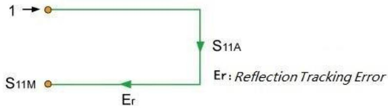
Figure 3-3 Open-circuit response calibration (open-circuit response)
