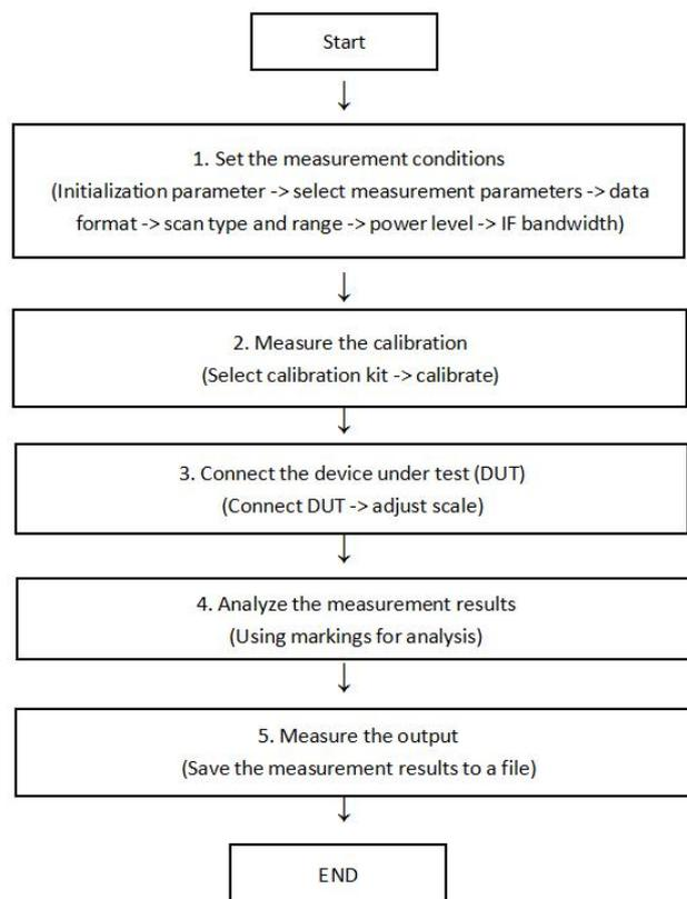
Figure 1-7 Basic test operation flow
