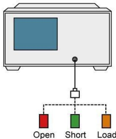
Figure 3-12 Full 1 port calibration - DUT connection diagram
