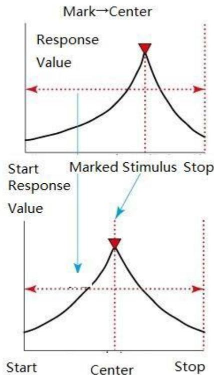
Figure 5-18 Marker Transfer --- Marker -> Center Function
