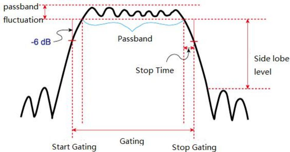
Figure 5-31 Time-domain gated measurement - Gated shape parameter definition
