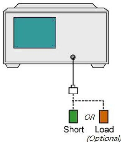
Figure 3-6 Short-circuit response calibration - DUT connection diagram
