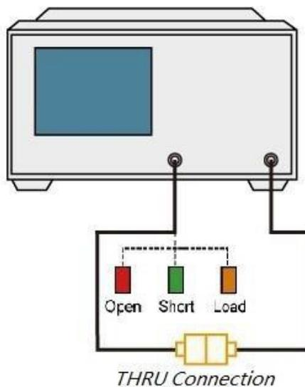
Figure 3-13 Full 2-port calibration - DUT connection diagram
