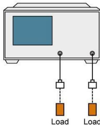
Figure 3-10 Transmission Response Calibration (Isolation Calibration) - DUT Connection Diagram
