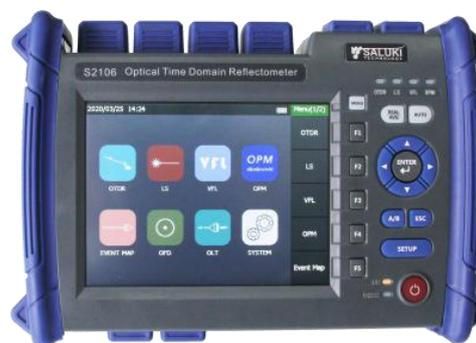
Saluki S2106P PON Optical Time Domain Reflectometer is a high performance multi-function test instrument designed for the FTTx network. The product has a range resolution of up to 0.05m and a ultra-short event blind zone of 0.8m. This product is designed for PON network testing.
