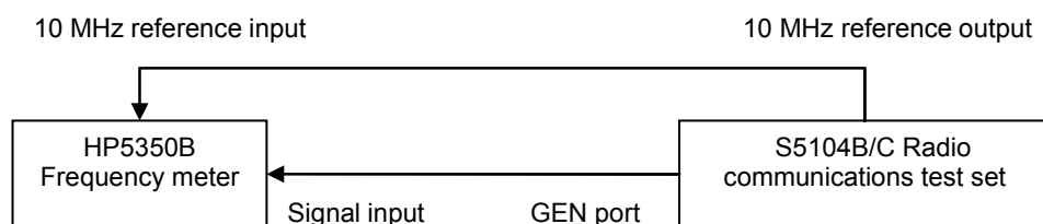
Fig. 6-7 Block diagram for RF signal generation frequency characteristics test
