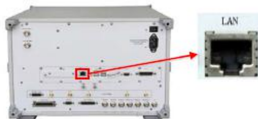
Fig. 2.7 LAN Interface of Rear Panel of Instrument
