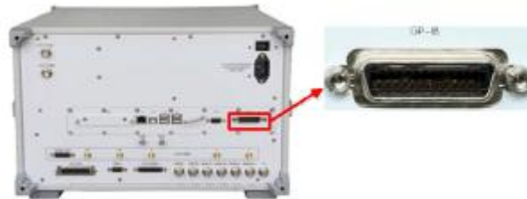
Fig. 2.10 GPIB Interface of Rear Panel of Instrument
