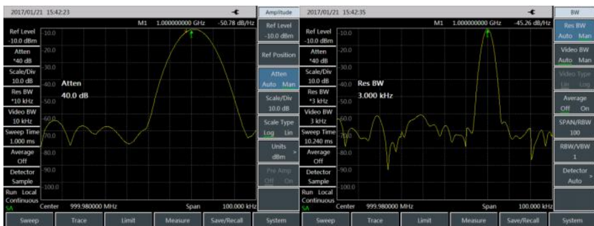
Fig. 4-11 Noise Measurement by Noise Marker Function
