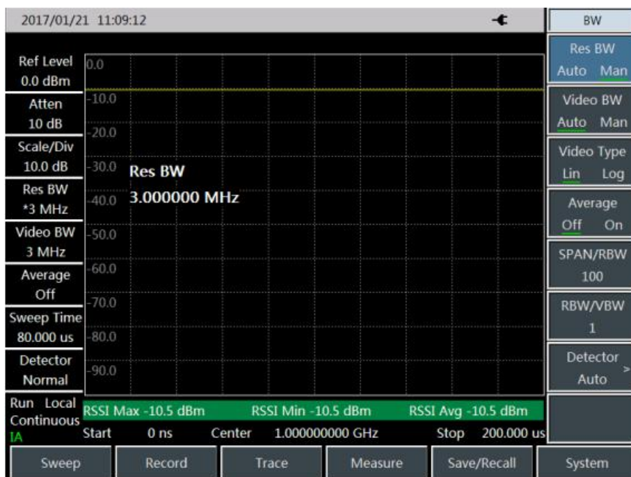
Fig. 5-2 RSSI Test Diagram of Interference Analyzer
