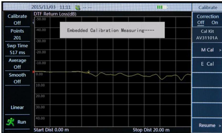
Figure 4-5 Start to Perform Embedded Calibration
