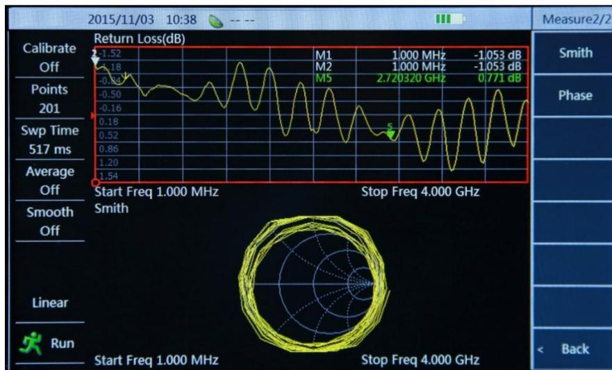
Figure 5-16 Simultaneous Display of Two Data Formats
