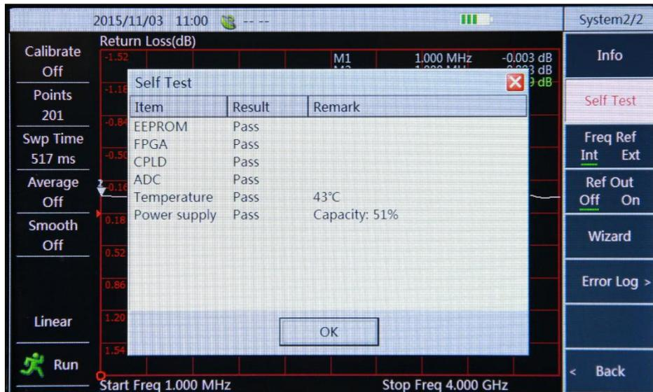
Figure 9-17 Self-test of Instrument
