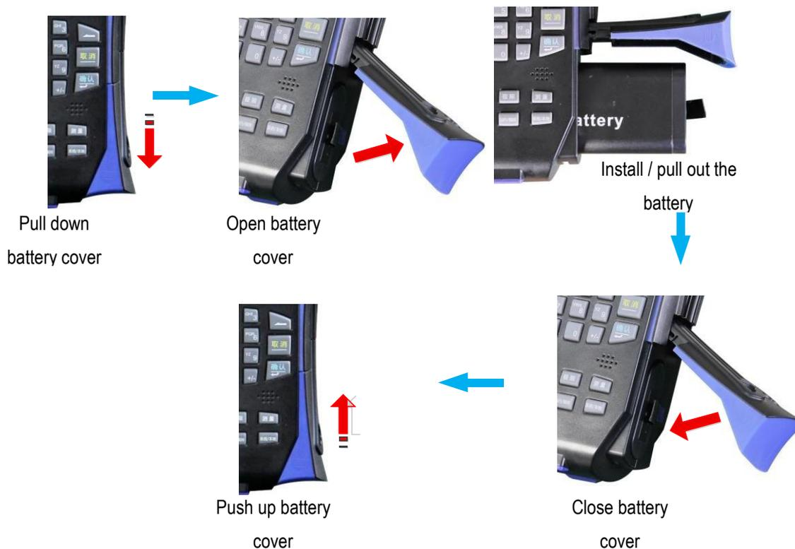
Figure 3-17 Battery Installation or Replacement Procedures
