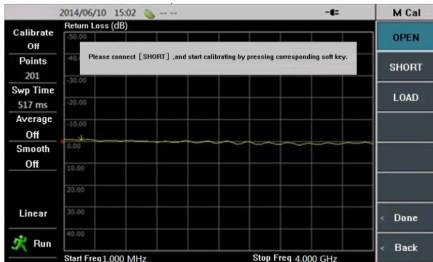
Figure 4-2 Calibration Short Standard
