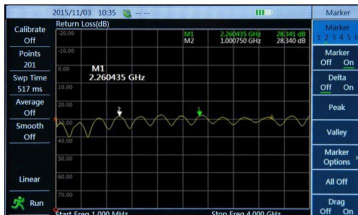
Figure 5-12 Marker Switch & Setting
