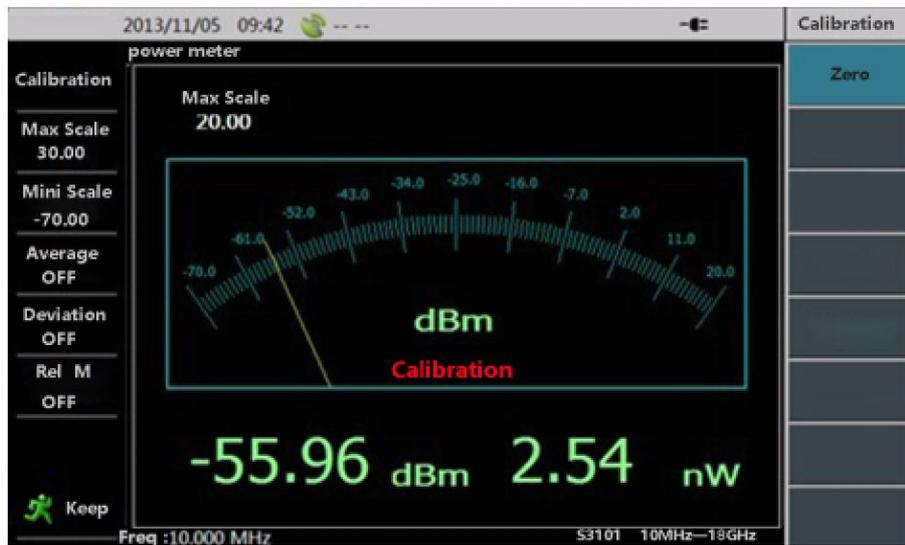
Figure 10-7 Power Meter Calibration
