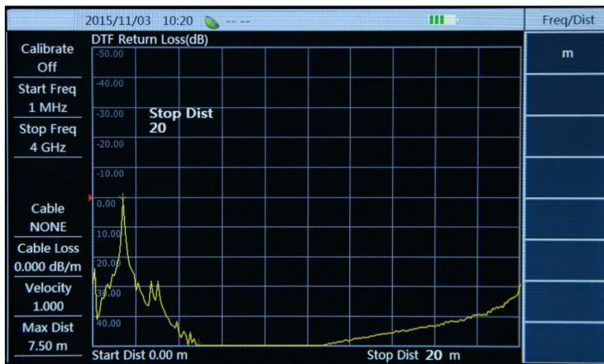
Figure 6-3 DTF Return Loss Measurement
