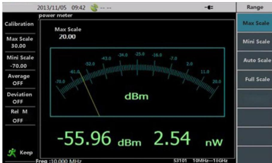
Figure 10-6 Amplitude Setting
