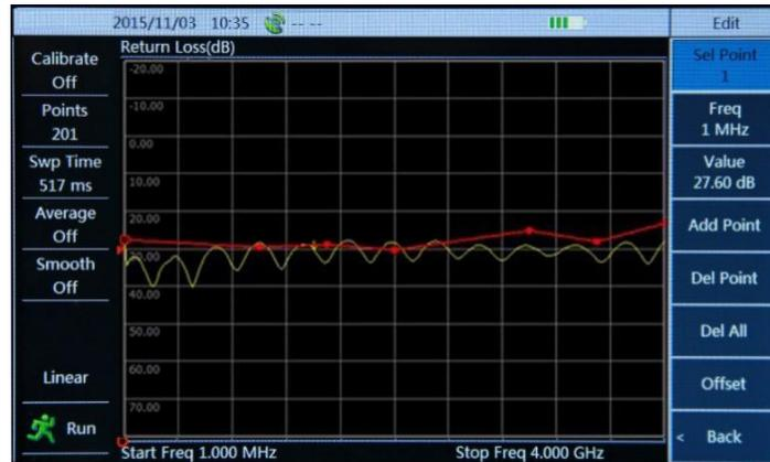
Figure 5-11 Limit Test
