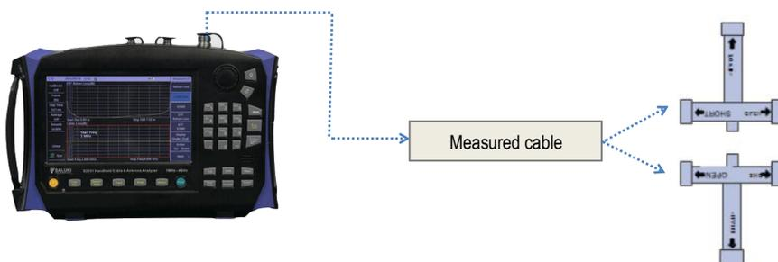
**Figure 3.7 Cable Loss Measurement Connections**
