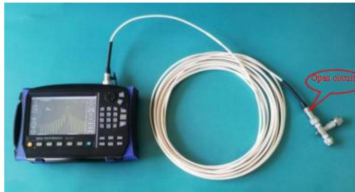
**Figure 3.10 DTF Return Loss Test Connection Diagram**
