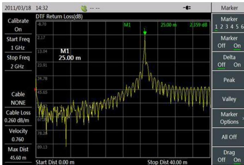
**Figure 3.11 Measurement on Length of Cable**
