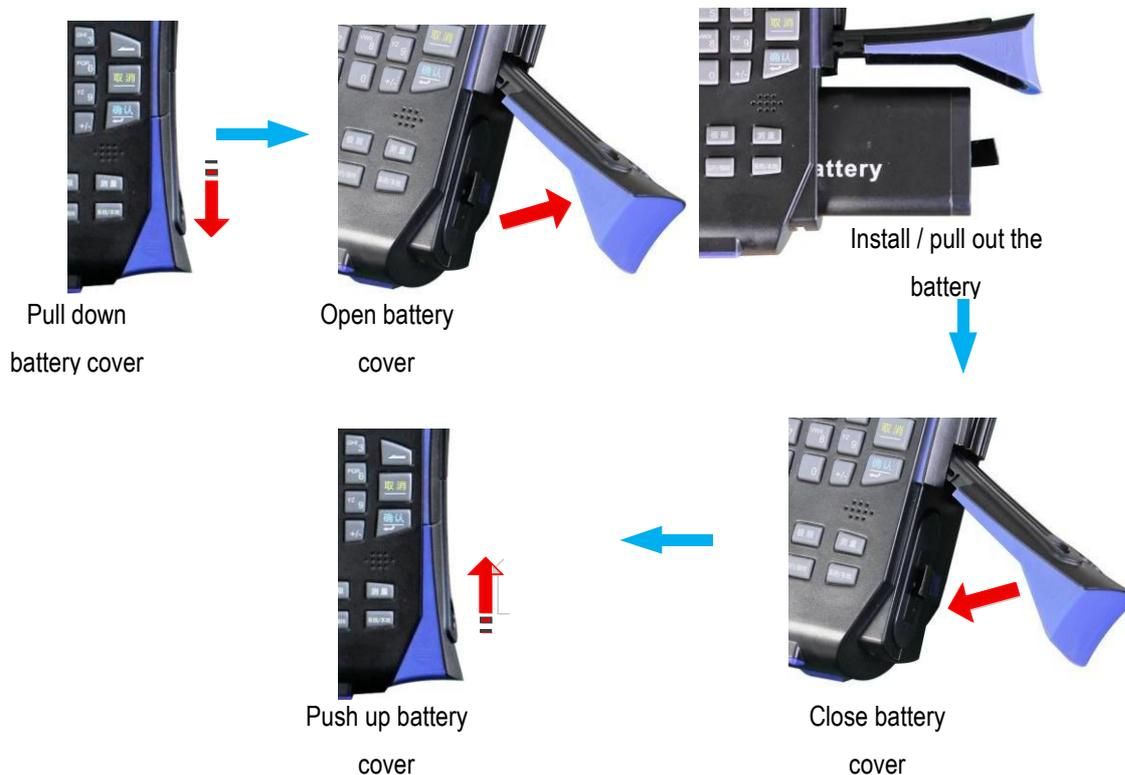
**Figure 2.7 Battery Installation or Replacement Procedures**
