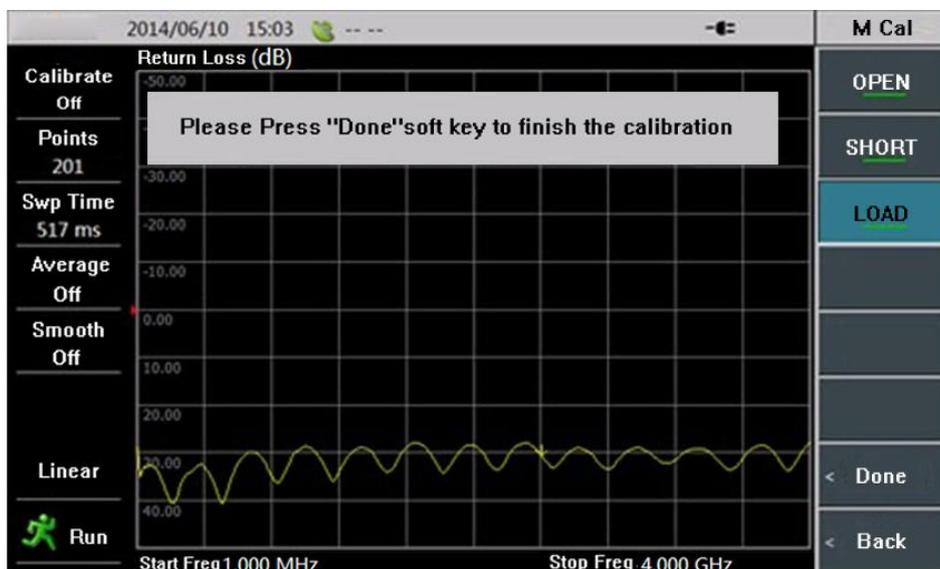
Figure 3.3 Complete Mechanical Calibration
