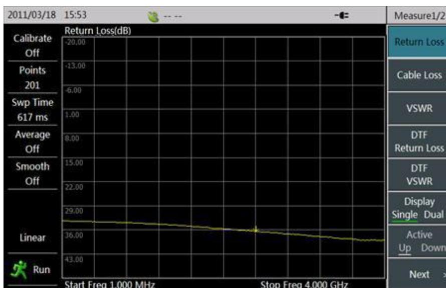
Figure 3.15 Return Loss Test of 10dB Attenuator
