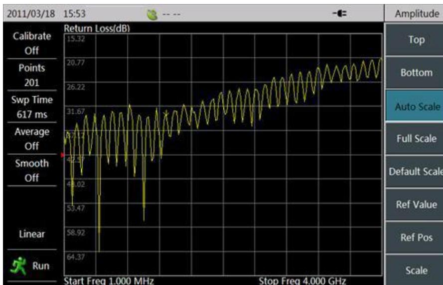
Figure 3.17 Return Loss Curve after Automatic Ratio Adjustment
