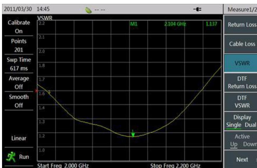
Figure 3.13 VSWR Test of Terminal Antenna TZD-P021Z05-195
