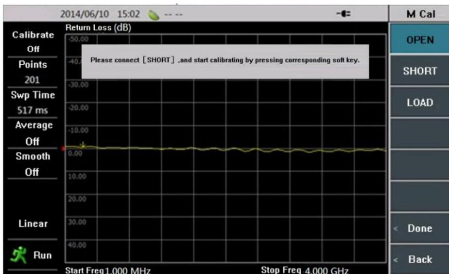
Figure 3.2 Calibration Short Standard
