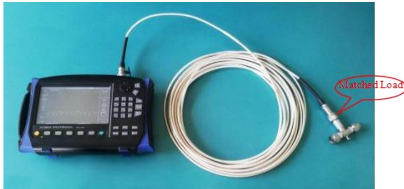
**Figure 3.6 Return Loss or VSWR Test Connection Diagram**
