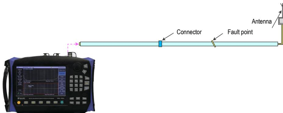
**Figure 3.9 DTF Measurement Connection**
