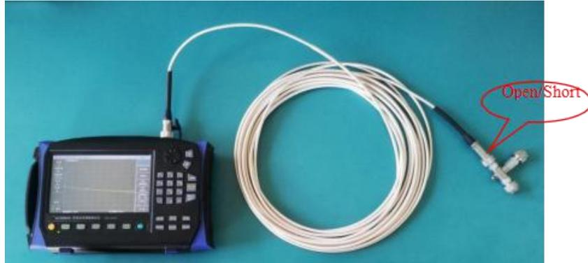
**Figure 3.8 Cable Loss Test Connection Diagram**
