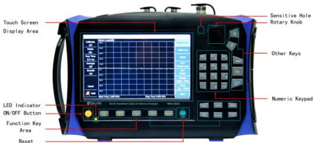
Figure 2.1 Front Panel of S3101 Cable & Antenna Analyzer
