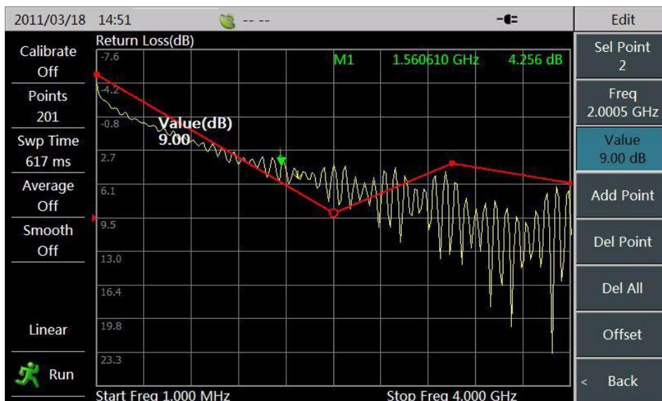
Figure 3.19 Alarm for Limit Line When Overstepping the Boundary
