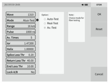
■ Measuring wavelength (nm): Set the test wavelength of OTDR.
