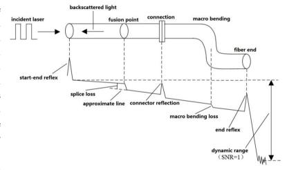
occurring at the junction between OTDR and the connector of the optical cable. This also includes the internal reflection of the instrument, and the loss and reflection between the connecting points cannot be detected in the near-end reflective area.
