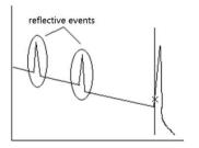
reflected signal. On the OTDR test curve, there is an upward spike signal with a certain width. The width and amplitude of the spike are mainly determined by the pulse width used in the test and the reflected intensity.
