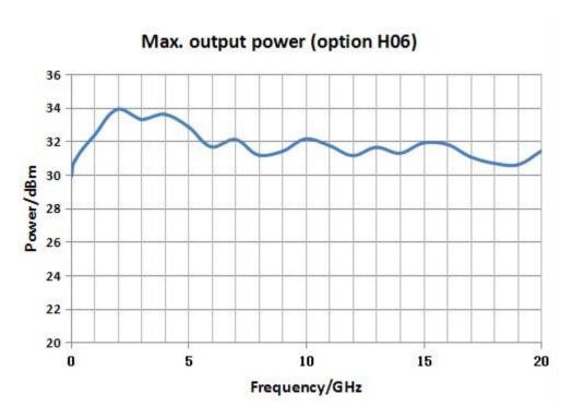
Fig.3.2 Max. Output Power of S1465D+H06
