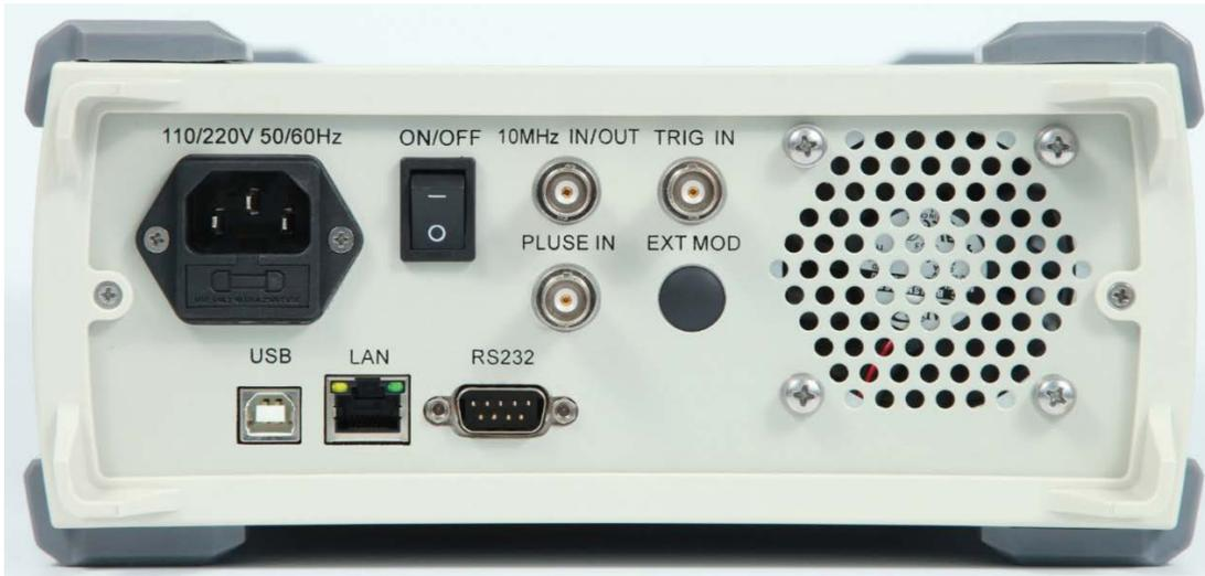
Figure 4-2 S1131 Signal Generator Rear Panel
