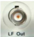
LF Out port is a 50ohm SMA port. It is used to output low frequency signals in different waveform.
