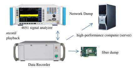
RF signal streaming and playback analysis function
